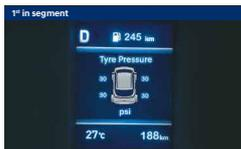
Tyre pressure monitoring system (TPMS) - highline
